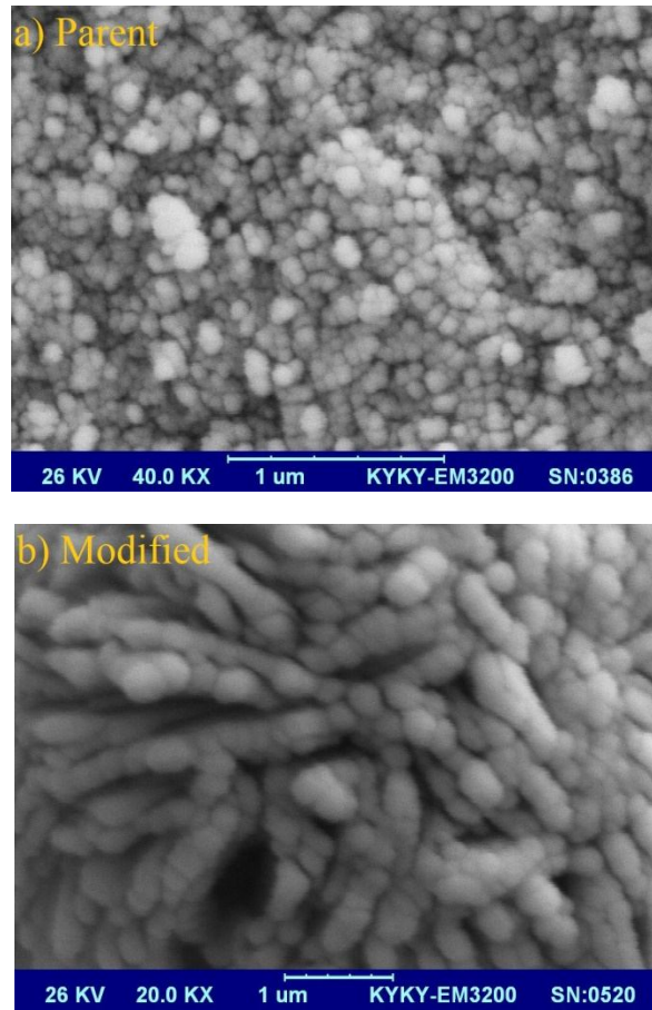
Fig. 4. FE-SEM image of the (a) parent, and (b) modified nano-adsorbent.
