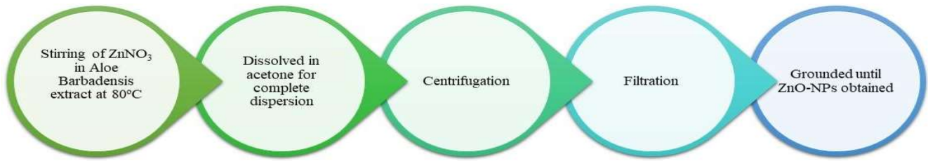
Fig. 1. Design Process of ZnO-NPs preparations through green synthesis route.
