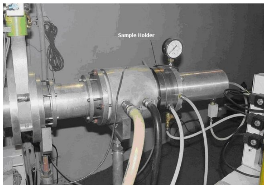
Fig. 1. Device for proton irradiation of PVB films.
