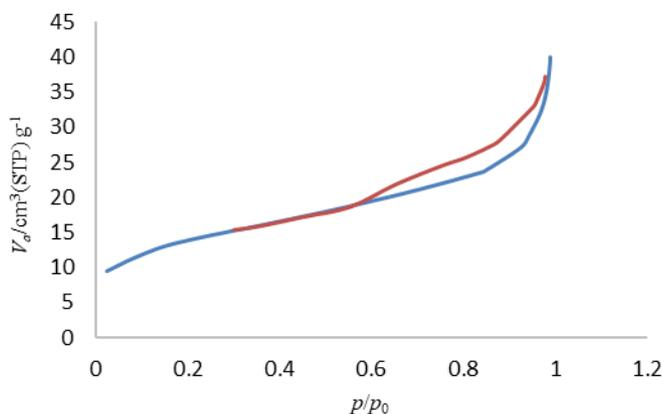
**Fig. 5.** The N<sub>2</sub> adsorption-desorption isotherm of perlite-calcium alginate-activated carbon.
