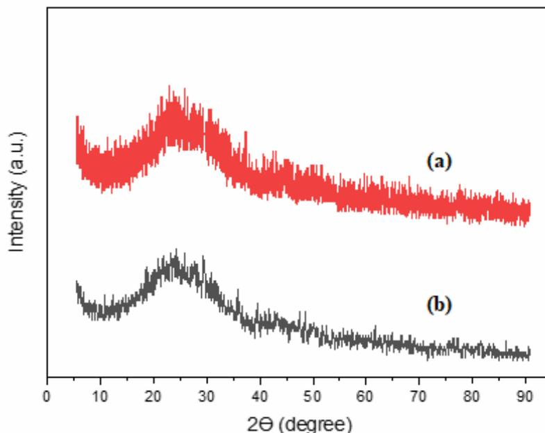
**Fig. 3.** XRD patterns of (a) the neat perlite and (b) perlite-calcium alginate-activated carbon.
