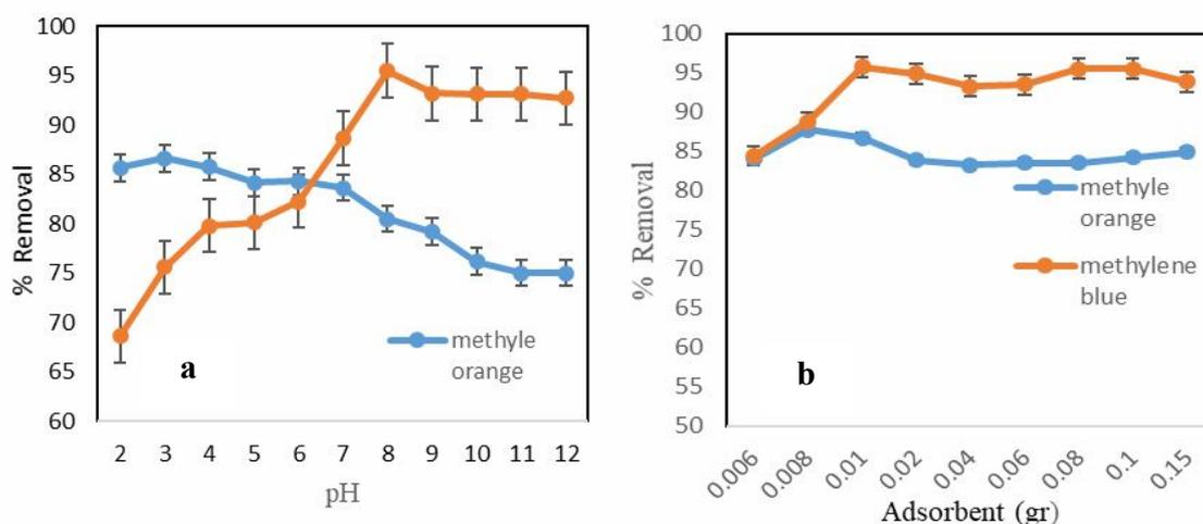
**Fig. 6.** The effects of (a) pH and (b) adsorbent doses for MB and MO adsorption on PCA.
