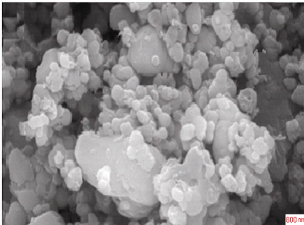
Fig. 2. The SEM image of LiMnPO<sub>4</sub> sample synthesized by solvothermal method.
