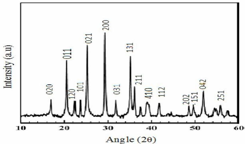
Fig. 1. XRD patterns of as-prepared LiMnPO<sub>4</sub> material.
