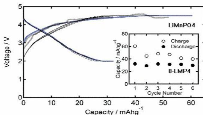
**Fig. 3.** The initial charge/discharge curves of LiMnPO<sub>4</sub>/C samples at current density of 0.02 mA cm<sup>-2</sup> in voltage range of 2.5-4.5 V and Cyclability of LiMnPO<sub>4</sub>.
