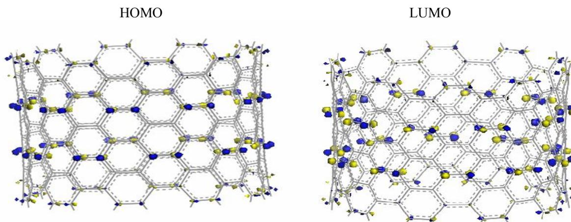
**Fig. 4.** The HOMO and the LUMO for the CNT (10,10) in gas.
