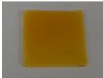
Fig. 1. Synthesized epoxy coatings. The sample contains 40% oleic acid that was used for enzymatic degradation.
