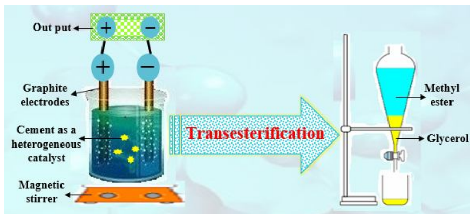
Fig. 1. A schematic of the process to produce biodiesel through electrolysis method.
