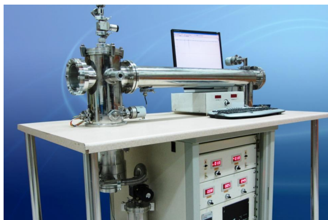
Fig. 4. Photograph of the time-of-flight mass spectrometer, constructed in Isfahan University of Technology.
