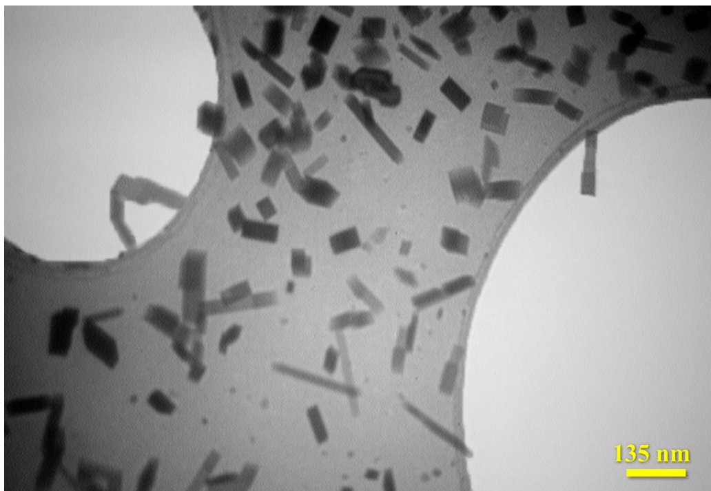
Fig. 3. TEM image of the as-prepared FeCe nanoparticles.
