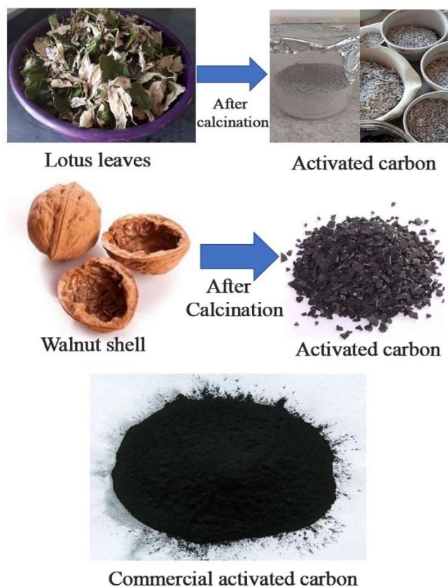
Fig. 1. Images of the adsorbents used in this work.
