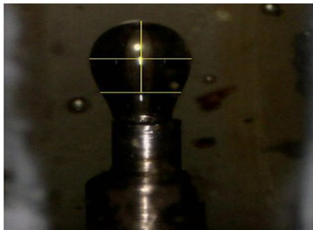
**Fig. 3.** An image of the oil drop in the high-pressure IFT device.
