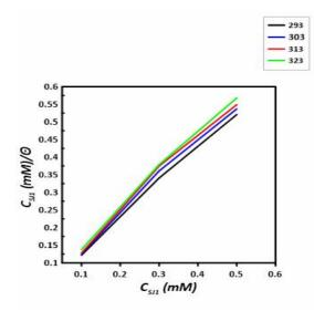
**Fig. 2.** Langmuir isotherm plot of SJ1 adsorption onto carbon steel surface in a 0.1 M HCl solution, at the range of temperatures (292-323) K.
