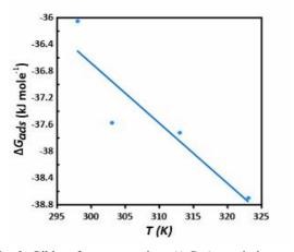
Fig. 3. Gibbs free energies ( $\Delta G_{ads}$ ) variation with temperature for SJ1 adsorption onto carbon steel surface in a 0.1 M HCl solution.
