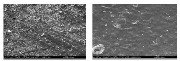
Fig. 8a-b. SEM for carbon steel in absence and presence of SJ1 inhibitor at 323K, (a) for corroded and (b) for inhibited.
