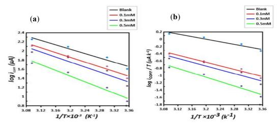
Fig. 4a-b. Arrhenius plots relationship for carbon steel corrosion in a 0.1 M HCl solution, in the absence and presence of various SJ1 concentrations at a range of temperature (293-323) K.
