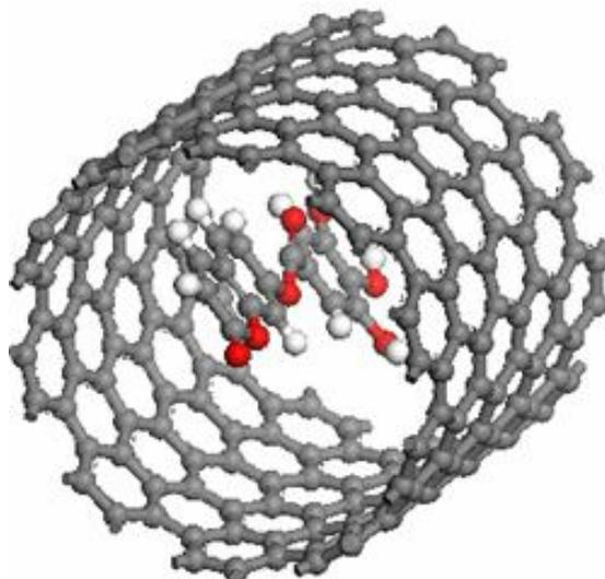
**Fig. 5.** Model for adsorption state for 1 molecule on the inner surface of a (10,10) single-walled CNT.
