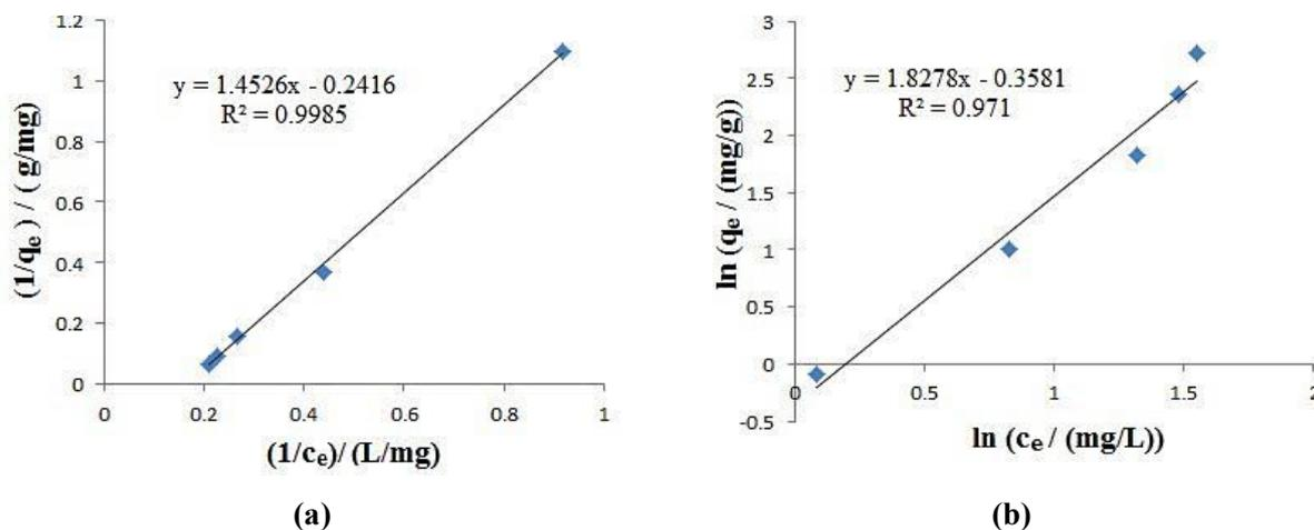
Fig. 6. The linearized Langmuir (a), Freundlich (b) isotherm of FA adsorption onto SWCNTs.
