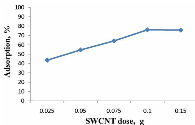
**Fig. 3.** Effect of CNTs dose on adsorption percentage: Initial FA concentration = 20 mg l<sup>-1</sup>, pH = 7, temp. = 25 °C, contact time = 60 min.
