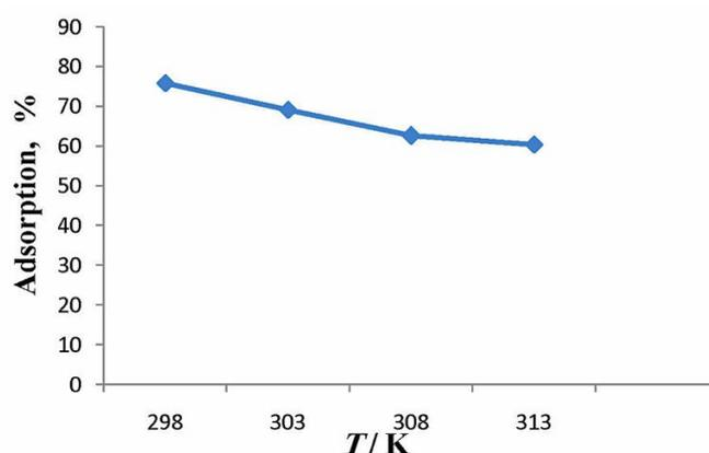
**Fig. 4.** Effect of temperature on percentage of adsorption: Initial FA concentration = 20 mg l<sup>-1</sup>, pH = 7, adsorbent dose = 0.1 g, contact time = 60 min.
