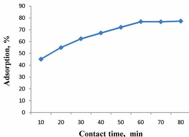
**Fig. 2.** Effect of contact time: Initial FA concentration = 20 mg l<sup>-1</sup>, pH = 7, adsorbent dose = 0.1 g, contact time = 60 min, and temp. = 25 °C.
