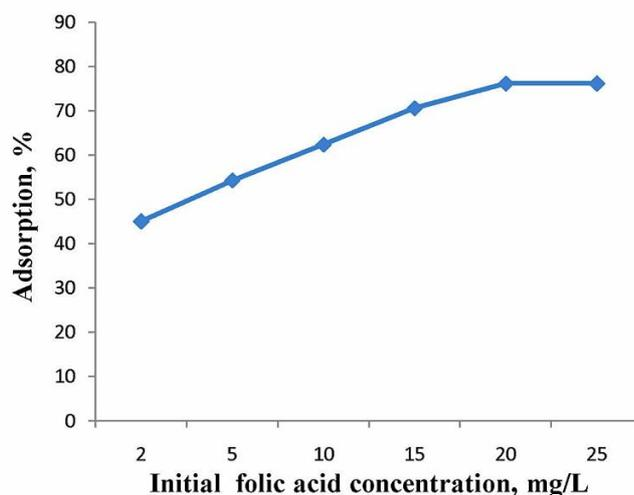
**Fig. 5.** Effect of initial FA concentration on percentage of adsorption: CNTs dose = 0.1 g, contact time = 60 min, temp. = 25 °C.
