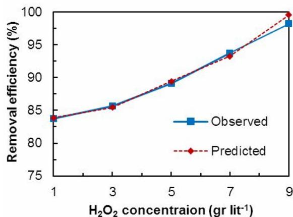
Fig. 3. Effect of H<sub>2</sub>O<sub>2</sub> concentration on mercaptan removal from the soil.
