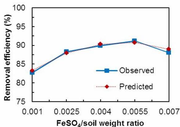
Fig. 4. Effect of FeSO<sub>4</sub>/soil weight ratio on mercaptan removal from the soil.
