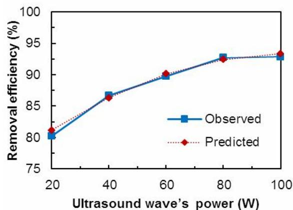
Fig. 5. Effect of ultrasound waves power on mercaptan removal from the soil.
