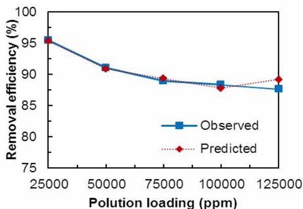
Fig. 6. Effect of pollution loading on the mercaptan removal from the soil.
