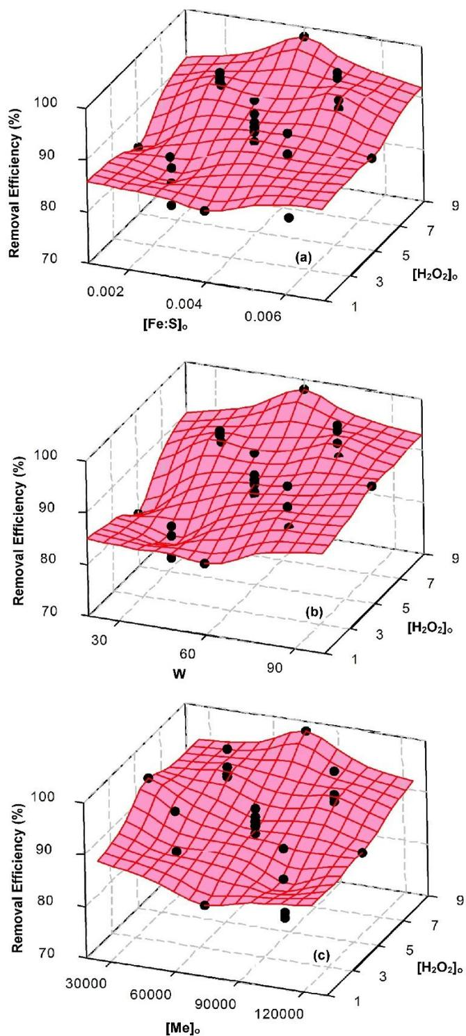
**Fig. 1.** Surface plots for TBM removal efficiency *versus*  $H_2O_2$  initial concentration and (a)  $FeSO_4$ /soil weight ratio, (b) ultrasound waves power, and (c) pollution loading (black points represent the experimental results).
